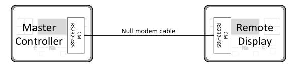
It is necessary to use CM-RS232-485 communication module on both the Master controller and the Remote display. COM 1 communication channel is used with these settings:
