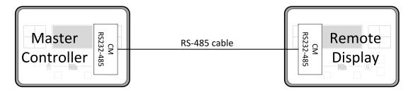
Any combination of internal RS485 port or external one on CM-RS232-485 communication module can be used for the Master and Remote Displays.
